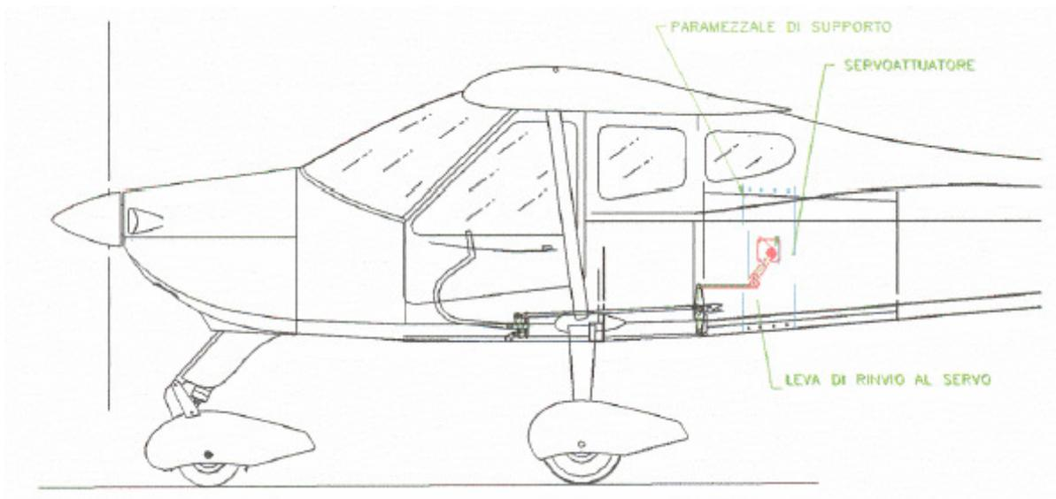
Figure 6: Stabilator actuator installation
