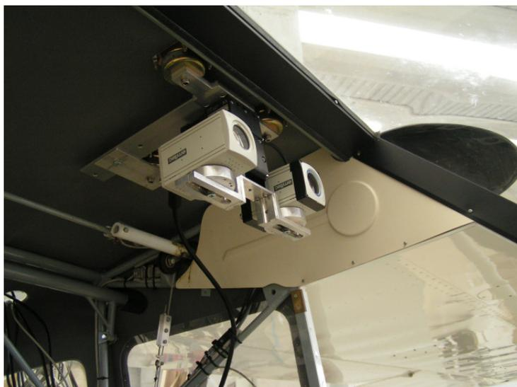
Figure 15: Stereoscopic cameras installation
