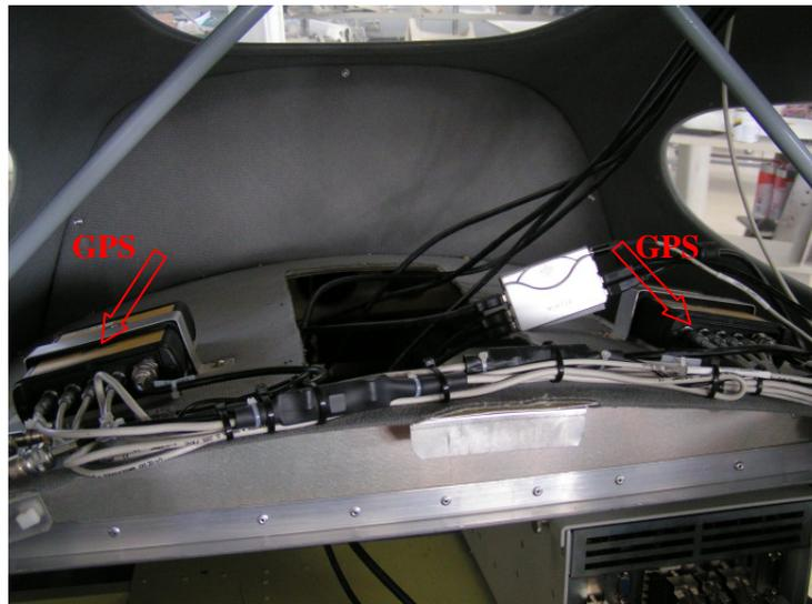
**Figure 10: GPS installation**
