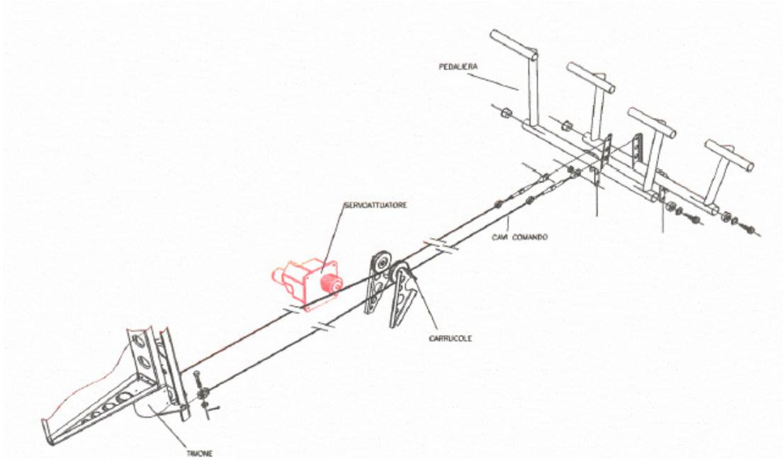
Figure 5: Rudder actuator installation
