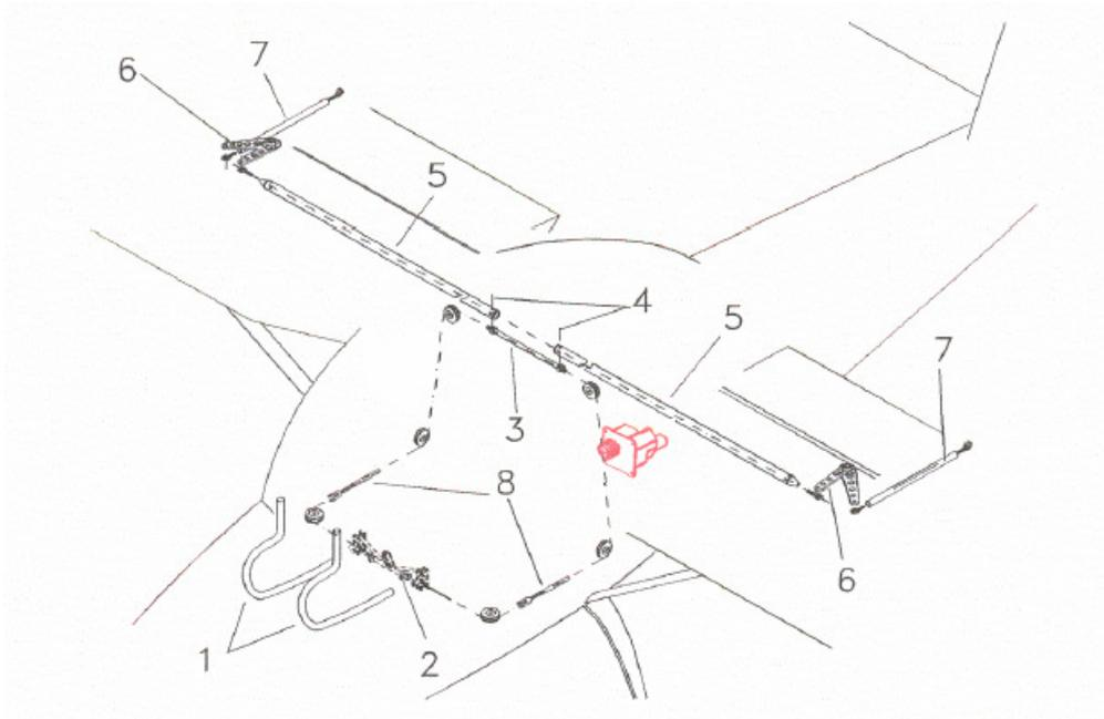
Figure 7: Ailerons actuator installation
