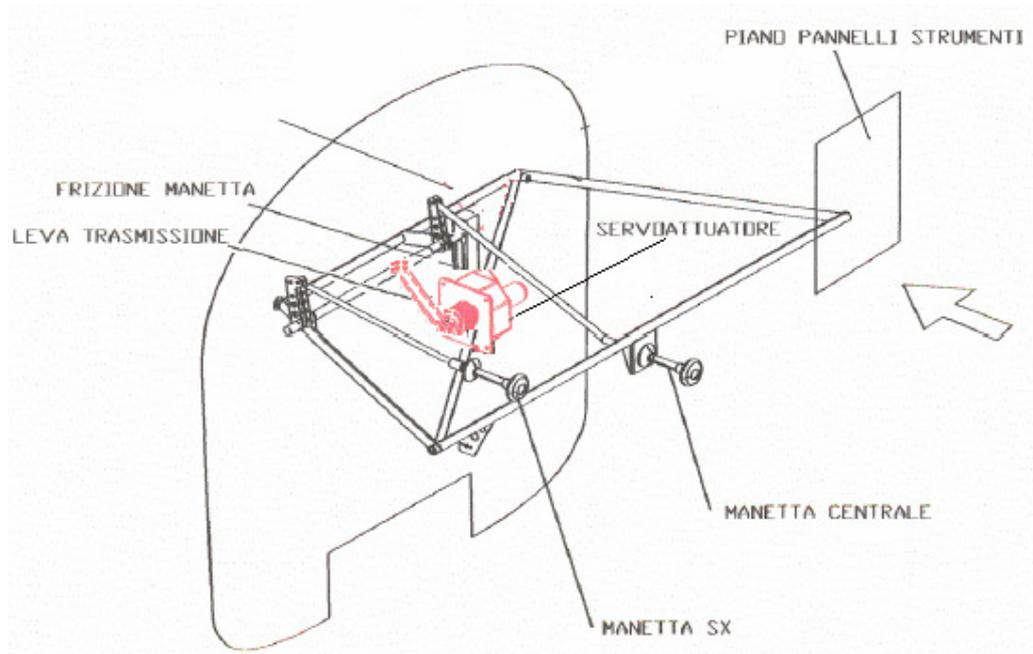
Figure 8: Engine throttle actuator installation
