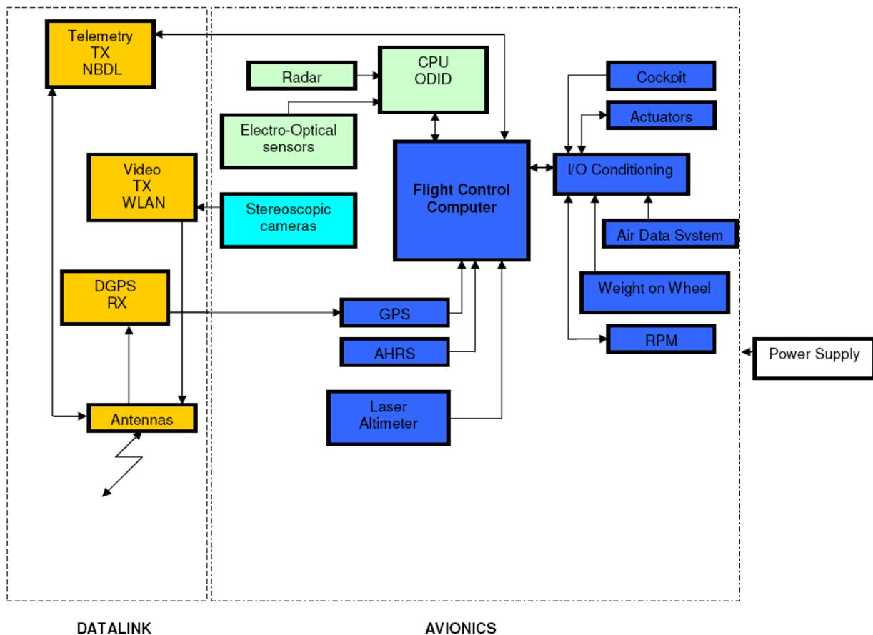
Figure 3: FLARE on-board architecture
