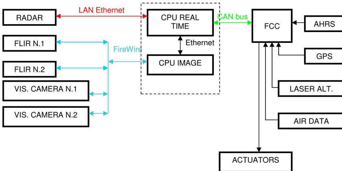
Figure 14: ODID hardware architecture
